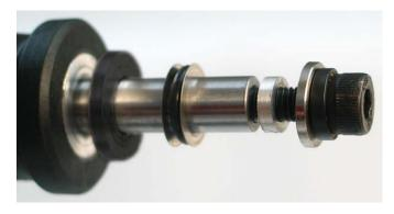
Select a set of two large black delrin delta rings and two small aluminum delta rings of matching thickness. The thicker the ring the more delta effect you will get. It's recommended to start with the thick set. Install the large rings facing the yoke then the shim, o-ring and shim from the EVO kit.
