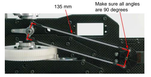
Insert the top servo between the frames following the steps indicated in the next 4 pictures.
