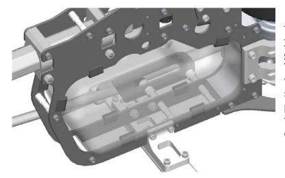
Place an M3 Washer on theM3x40mm screw and pass it through the boom support end and the 7mm spacer. Install the plate and a 17mm spacer in the back hole as well as a M3x25mm screw and 17mm spacer in the front hole. Using blue loctite install the assembly in place.
