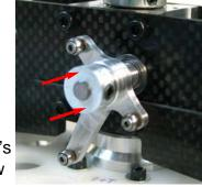
Notice that the setscrews are not cup but flat bottomed. This allows the lever to selfalign to the flats when tightened. If they are ever replaced remember to use flat bottom setscrews or the levers won't be truly aligned to each other.
