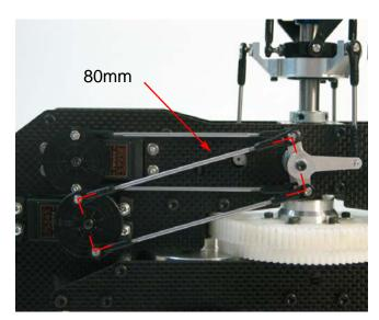
Install two *Hirobo ball links* on two 80 mm long pushrods and adjust them to match the distance between the servo wheel center and the lever's center of rotation. Install them as in the picture to the left and make sure there is a 90 degree angle between the rod and a line between the ball links and the centers of rotation.
