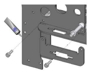
There are two places to install switches in the Avant EFX. There is one on the receiver/battery plate for a switch that can be accessed from the bottom and one in the optional switch plate that can be accessed from the side. There are some servo system that use a switch for the receiver battery and another one for a 7V high voltage servo system.
