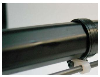
Using blue loctite screw each end of the cured pushrod threads as shown on the picture to the left.
