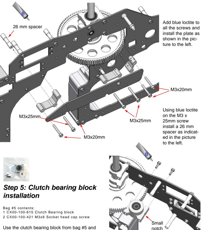
Use the clutch bearing block from bag #5 and install it with the provided screws as indicated in
