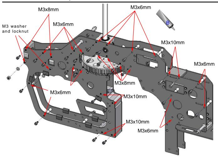
Using blue loctite install sixteen (16) M3x6mm screws in the locations marked with the arrows. Using blue loctite install six M3x8mm screws in the locations marked with arrows or with a blue dot if you are looking at the color version.
