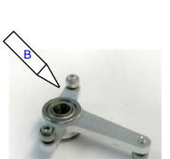
From *Bag #11* select the CCPM shaft. Using blue Loctite Install the M2.5x8 screw and M2.5 flat washer at the end of the shaft as shown in the picture.
