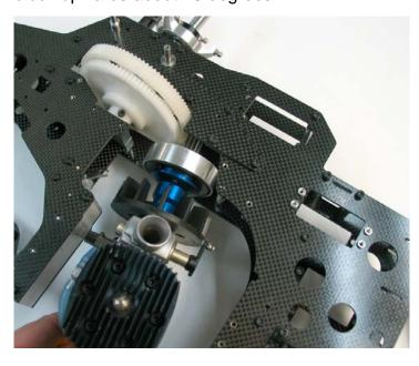
Insert the engine with the clutch stack installed into the clutch bearing block.
