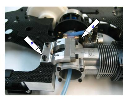
Add blue loctite to all the clutch bearing block screws and tighten them in place.
