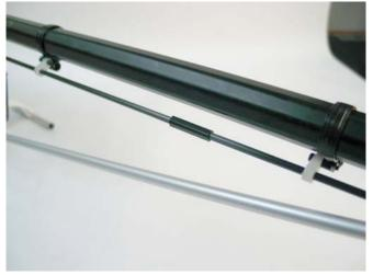
crank arm and tail control arm match the ball link's centers. Let the J-B Weld cure overnight. Once the J-B Weld has cured if additional fine tuning is necessary it can be done by screwing the ball link inward or outward as required.
