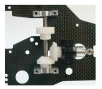
As shown on the picture to the left those using the *Hirobo torque tube system* won't need to install the sleeve.
