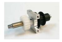
Slide the bearing block with the bearing opening facing the *tail pulley*. Install the *tail pulley* and slide the pin in place with a set of pliers as indicated on the picture to the left. Install the *brass sleeve* on top of the gear. If you're using 8.08 gear ratio then don't install the sleeve and read the special 8.08 ratio instructions and notes on the next page.
