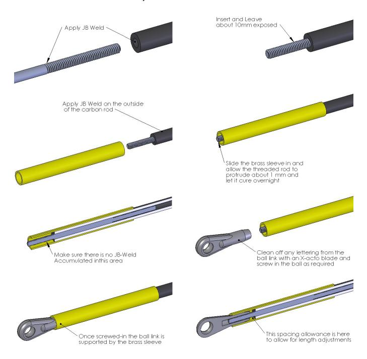
Install one sleeve in the front of the rudder pushrod at the X-Lever and one in the back at the tail pitch lever.
