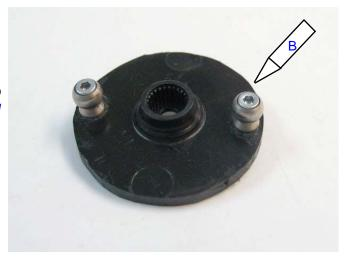
Install the wheel on the servo and make sure the ball face inward towards the left frame. If the screws protrude above the 2mm nuts file them to make them flush with the nuts.
