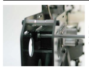
Secure the servo with four M2.5x10mm phillips round head screws and M2.5 washers. Screwdriver access to the inner side of the frame is provided through through holes or openings on the opposite side frame.
