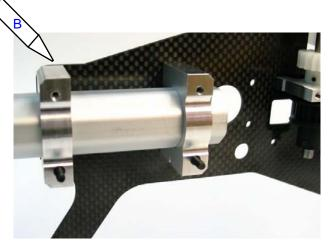
Using blue loctite install the boom clamps with two M3 x 8mm from bag #6. Slide the *Hirobo tailboom* between the two boom clamps to make sure they are aligned before tightening the screws. Make sure the threaded holes are pointing upwards and the through holes for the M3 x 35mm screws are
