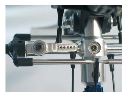
Install two *Hirobo ball links* at both ends of each one of the three 35 mm pushrods. install them in the ends of all the CCPM levers and install the other end in the balls of the swashplate as indicated in the picture below.
