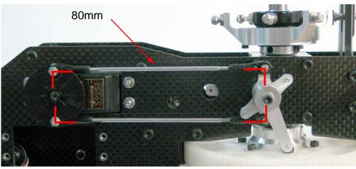
adjust them to match the distance between the servo wheel center and the lever's center of rotation. Install them as in the picture above and make sure there is a 90 degree angle between the rod and a line between the ball links and the centers of rotation.
