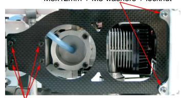
Using Blue loctite Install the plate using four M3x8mm screws for the four holes in the back of the plate. Install two M3 washers on two M3x12mm screws and insert them from the top through the bottom plate and through the front landing gear mount holes. Use another M3 washer and install an M3 locknut on each screw.
