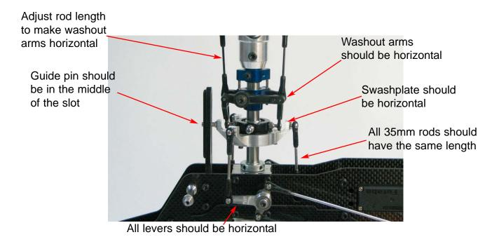
Reinstall the 35mm rods in place and make sure the swashplate is perfectly leveled. This should mean also that all levers are horizontally aligned.
