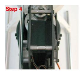
Trim the diameter of a servo wheel and install two Hirobo 2525-007 - 5MM Ball with stand, 2532-031 M2x6mm cap screw and 2mm nut on the REVERSE side of the servo wheel as shown in the picture to the right. Apply blue loctite when installing the 2mm nut.
