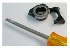
Using a flat screwdriver as a wedge insert a screwdriver into the slits as a wedge and rotate it to break the plastic outer casing off. as indicated in the pictures.
