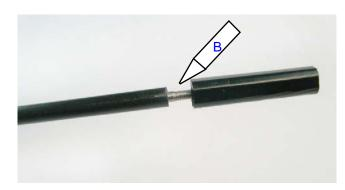
Install the other two 50mm threaded rods as explained before but this time leave about 20mm of the short threaded rod exposed. Install the ball links and then adjust the depth at which the threaded pushrod sits before it cures as required to make the rudder bell-
