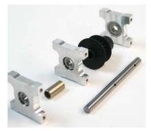
Notice the orientation of the tail pulley shaft bearing blocks. It's important to have them oriented in the correct facilities are that they existed to
