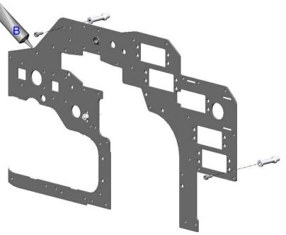
Flip over the left frame and using nine M3x6mm screws install the eleven 26mm cross members in the locations indicated in the picture to the left. Use Loctite when installing the screws.
