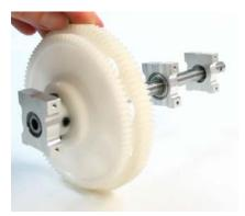
Install the main shaft into the *gear/clutch* assembly the same way the original hirobo shaft is installed. Notice which way the bearings are facing and slide the bearing blocks into the mainshaft as shown in the pic-
