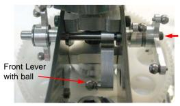
Install the M4 setscrew in the front lever. Pass the CCPM shaft assembly through the left frame's flanged 5 mm ID bearing and then through the Front lever and through the right frame's 5mm ID flanged bearing. Install the long ccpm shaft spacer and the Pitch lever as shown in the picture to the left.
