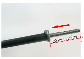
Using the M2.5mm screw install the pushrod guide on the *Hirobo 0414-137 control rod guide* as shown in the picture to the left. Use loctite and install the M2.5 plain nut in the end indicated in the picture.
