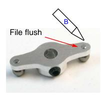
Once the Elevator lever balls are installed file the screw ends flush so that they clear the M3 socket heads from the left frames.
